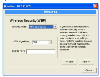
When "WPA-shared key", also named "WPA-PSK" requires users to select the advanced encryption methods, i.e. TKIP and enter a set of shared key.
